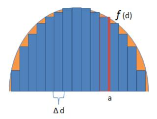
To determine the area of a rectangle, multiply its width ( $\Delta d$ , delta d) times its height (a, which is determined from either direct measurement or from the equation, f(d), which is short hand notation for the *function* of the curve), as shown in the illustration.
