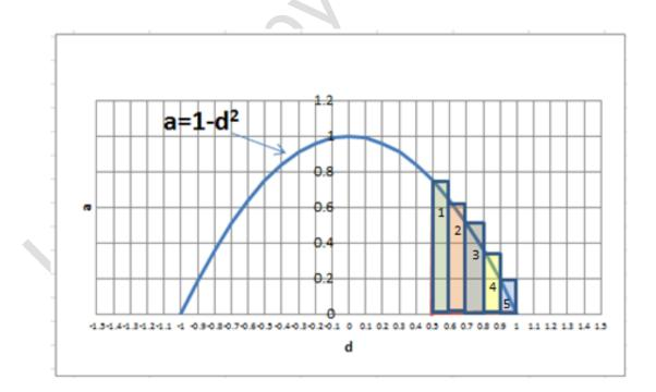
The height (a) of each outer rectangle is determined by the curve equation or function (f(d)) value for the selected *d* value.
