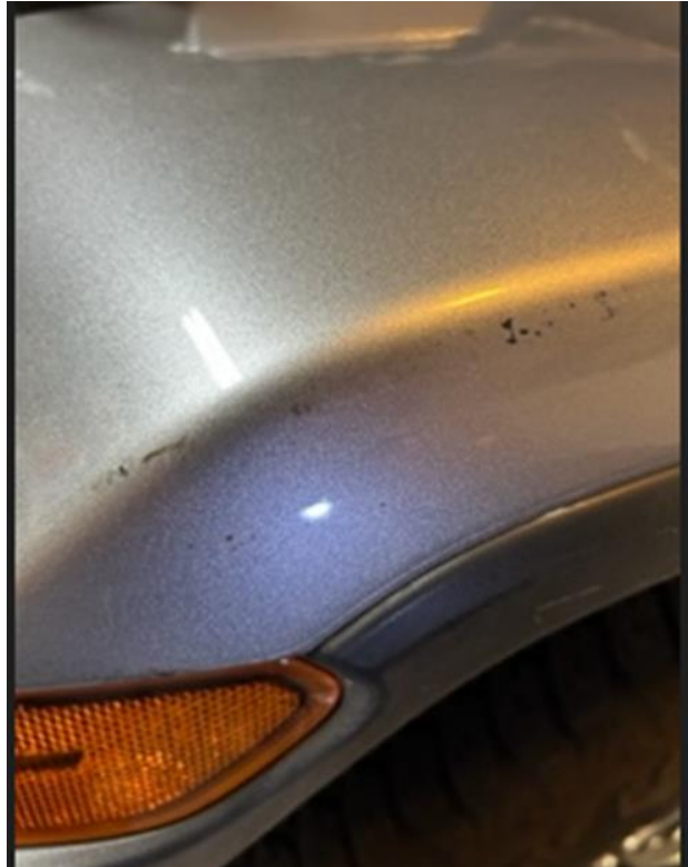
BODY PAINT DAMAGE CAUSED BY FLUTTERING/LOOSE FITTING COVER...
