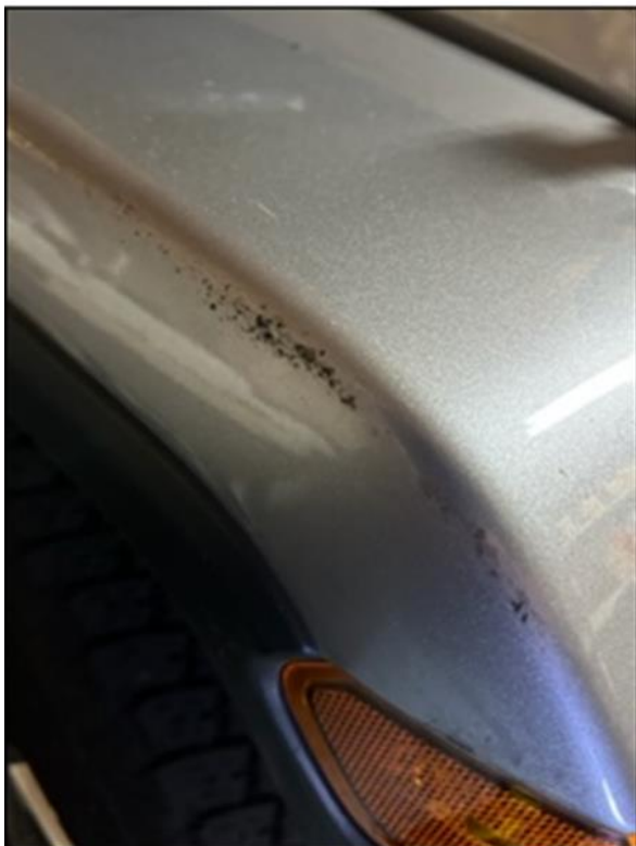
BODY PAINT DAMAGE CAUSED BY FLUTTERING/LOOSE FITTING COVER...
